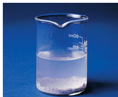
▲ \text{AgCl} does not dissolve in water; it remains as a white powder at the bottom of the beaker.
