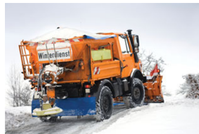
▲ In winter, salt is often applied to roads so that the ice will melt at lower temperatures.
