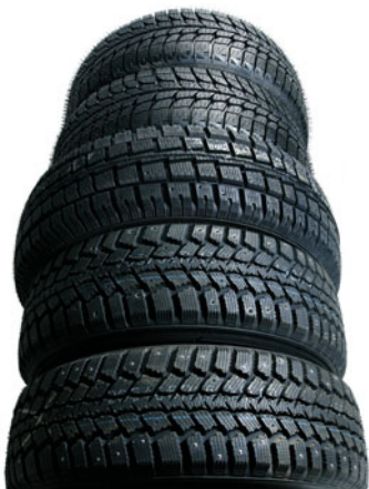
▲ Automobile tires are black because of the carbon black that is added to strengthen the tires and maintain flexibility.
