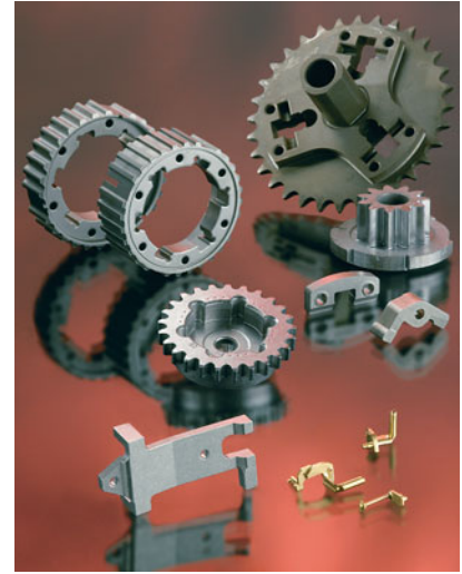
▲ These metal products were all made by powder metallurgy.
