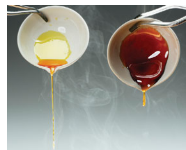
▲ Molten sulfur below 150 °C (left) and nearing 180 °C (right).
