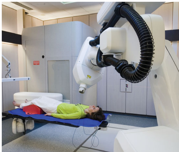
▲ FIGURE 19.19 Radiotherapy for Cancer This treatment involves exposing a malignant tumor to gamma rays generated by nuclides such as cobalt-60. The beam is moved in a circular pattern around the tumor to maximize exposure of the tumor to radiation while minimizing the exposure of healthy tissues.
