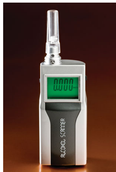
▲ FIGURE 18.19 Fuel-Cell Breathalyzer The fuel-cell breathalyzer works by oxidizing ethyl alcohol in the breath to acetic acid. The electrical current that is produced is proportional to the concentration of ethyl alcohol in the breath.
