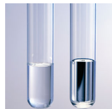
▲ FIGURE 11.22 Menisci of Water and Mercury The meniscus of water is concave because water molecules are more strongly attracted to the glass wall than to one another. The meniscus of mercury is convex because mercury atoms are more strongly attracted to one another than to the glass walls.
