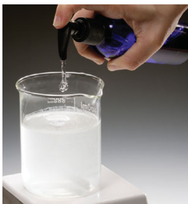
▲ FIGURE 12.19 A Colloid Soapy water is an example of a colloidal dispersion. The haze is due to the scattering of light by the colloidal particles.
