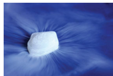
▲ Dry ice (solid \text{CO}_2 ) sublimates but does not melt at atmospheric pressure.
