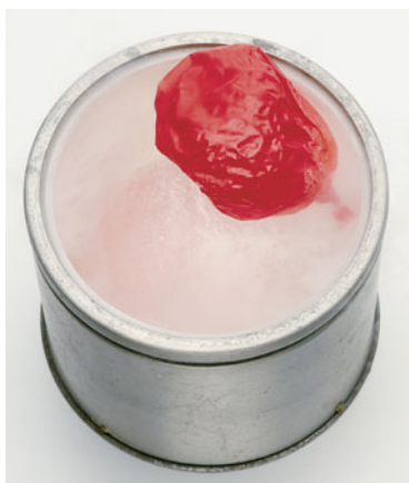
▲ If we place a balloon into liquid nitrogen (77 K), it shrivels up as the air within it cools and occupies less volume at the same external pressure.
