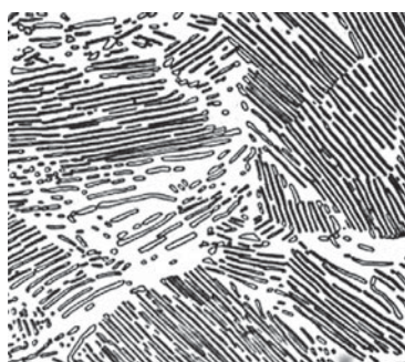
▲ This micrograph shows cementite (dark regions) in steel.
