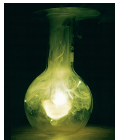
▲ FIGURE 8.19 Reaction of Sodium and Chlorine to Form Sodium Chloride.
