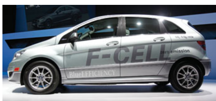
▲ The B-Class F-Cell vehicle from Mercedes Benz is a four passenger sedan that accelerates from 0 to 60 mph in about 9 seconds. The car runs on hydrogen and its only emission is water.
