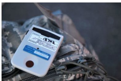
▲ FIGURE 19.7 Film-Badge Dosimeter A film-badge dosimeter consists of a piece of photographic film in a light-resistant container. The film's exposure in a given time is proportional to the amount of radiation it receives.
