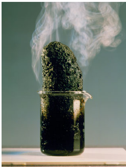
▲ FIGURE 22.26 Dehydration of Sucrose Sulfuric acid dehydrates sucrose by removing the hydrogen and oxygen as water molecules and leaving carbon behind. The porous carbon foam forms because the reaction is very exothermic.
