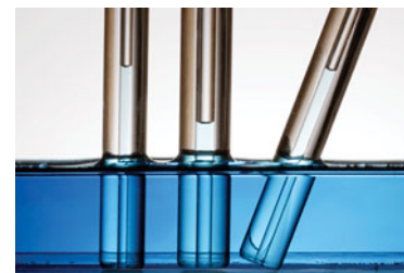
▲ FIGURE 11.21 Capillary Action The attraction of water molecules to the glass surface draws the liquid around the edge of the tube up the walls. The water in the rest of the column is pulled along by the attraction of water molecules to one another. As can be seen in this figure, the narrower the tube, the higher the liquid will rise.
