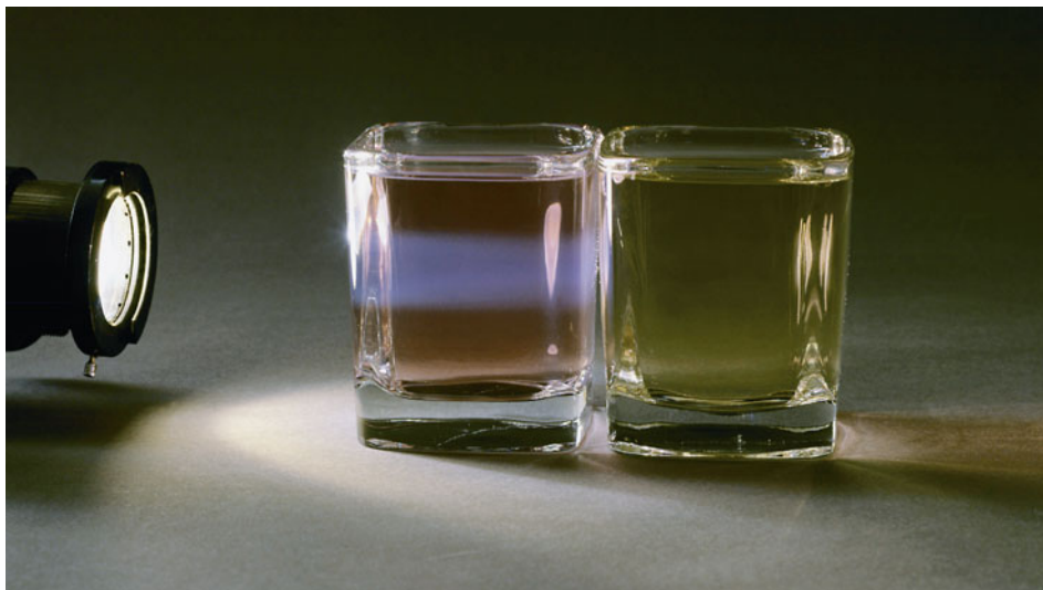
▲ FIGURE 12.23 The Tyndall Effect When a light beam passes through a colloidal suspension (left), it is visible because the colloid particles scatter some of the light. The beam is not visible in pure water (right), nor would it be visible in a noncolloidal solution.
