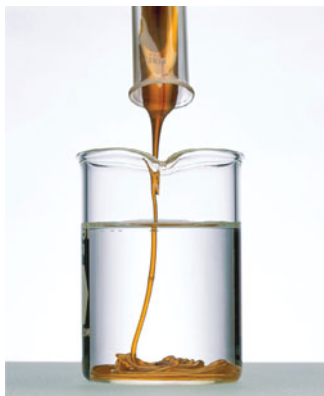
▲ FIGURE 22.25 Quenching Liquid Sulfur When hot liquid sulfur is poured into cold water, the sulfur quenches into an amorphous solid.
