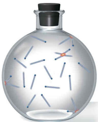
▲ FIGURE 5.15 A Model for Gas Behavior In the kinetic molecular theory of gases, a gas sample is modeled as a collection of particles in constant straight-line motion. The size of each particle is negligibly small, and the particles' collisions are elastic.
