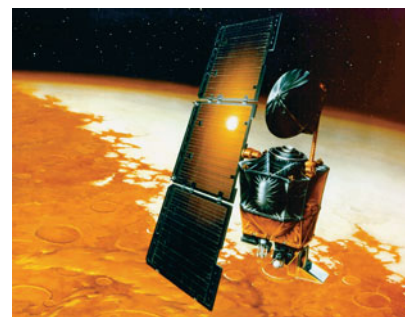
▲ The $125 million Mars Climate Orbiter was lost in the Martian atmosphere in 1999 because two groups of engineers failed to communicate to each other the units that they used in their calculations.
